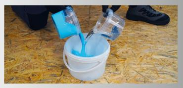
CN 94 is a **concentrate and can be easily diluted** with water. The ratio 1:3 is recommended but depending on the application surface (check the Technical Data for more detailed information). The product has a wide temperature range of application above 5°C.
